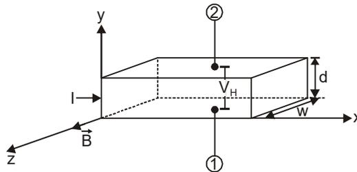
**Case-II :** If the given specimen is of p-type semiconductor, then event will be carried by holes. Hence in this case face-(1) will become positively charged with respect to face-(2). Hence Hall voltage  $V_H$  will be (-)ve.
