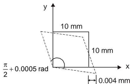
If the shear strain  $\gamma_{xy}$  at this point is expressed as  $0.001 k$  (in rad.) the value of  $k$  is
