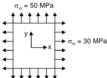
The Young's modulus of the material is  $2 \times 10^{11}$  N/m<sup>2</sup> and the Poisson's ratio is 0.3. If  $\sigma_{zz}$  is negligibly small and assumed to be zero, then the strain  $\epsilon_{zz}$  is
