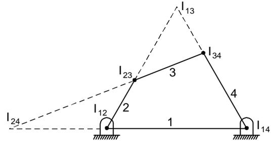
**Q-3:** One of the turning pairs of a four-bar chain is replaced by a sliding pair. Draw the inversions by fixing different links. Give one application for each of the mechanism. [10 Marks ESE-2013]
