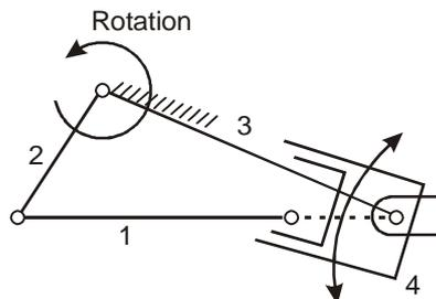
Here link-2 rotates (i.e., crank) and cylinder-4 oscillates. The piston is fixed at the end of link 1 which reciprocates in cylinder.
