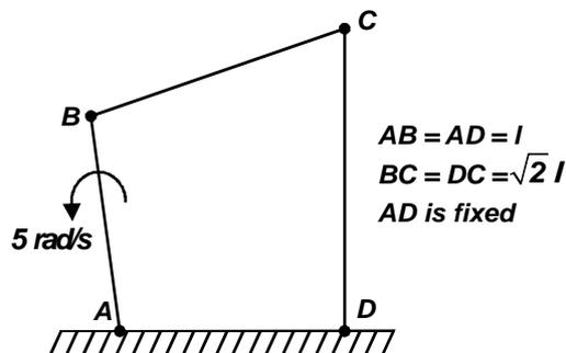
The driver link AB of a four bar mechanism is rotated at 5.0 rad/s in counter clockwise direction as shown in the above figure. Locate and indicate the Instantaneous Centre (I.C.) of the coupler BC with respect to fixed link AD at an instant when  $\angle BAD = 180^\circ$ . Find angular velocity of the coupler using I.C. method only. [2 Marks ESE-2010]
