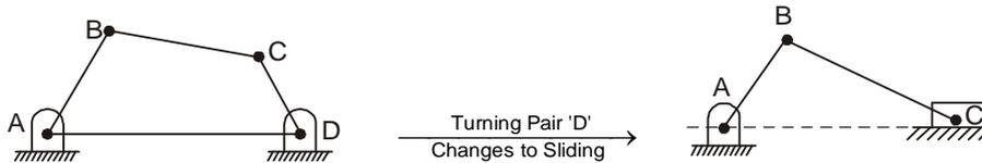
**Various inversion of sliding pair mechanism.**
